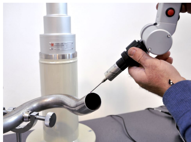
Pipe measurement by touch probe
