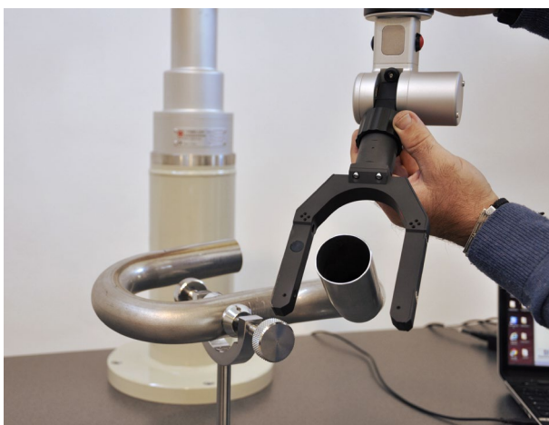
Pipe measurement by laser fork
