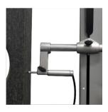
**Perpendicularity** Squareness measurements with electronic probe (V6)
